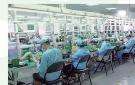
DIP through-hole assembly
