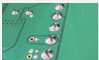
Smooth & Plump Solder Joints
