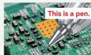
Precision Component Mounting(01005)
